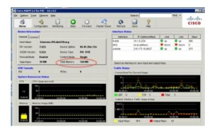
The device takes PC 100 CL2 SDram memory modules. To save money you can use any compatible memory with these specs and (saving a couple of hundred dollars off what Cisco charges for same part). Although you can theoretically add more memory such as 256 megs – I choose not to since we are using a Restricted license – the software will not use more than 128 megs of RAM (UR license allows 256 on software 7.x or higher).
